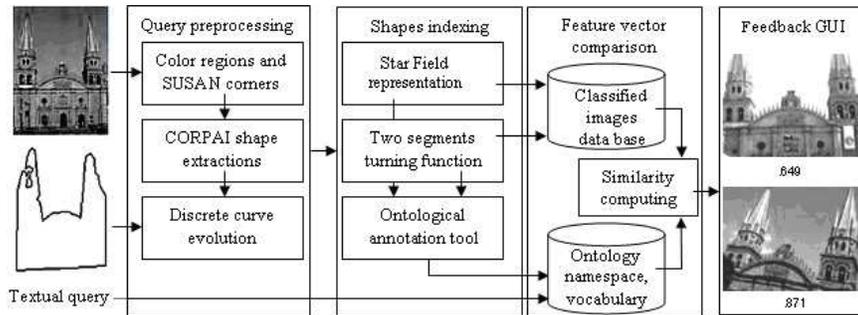
Figure 4. Block diagram of the proposed IRONS system
